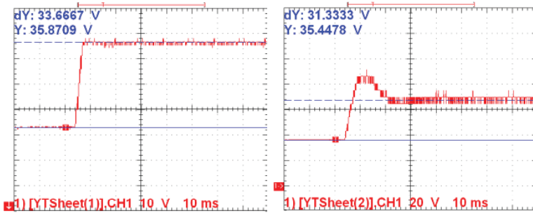
(a) SMC voltage from load to no-load on arc welding (b) PI control voltage from load to no-load on arc welding
